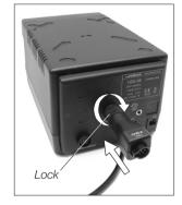
2. Connect the tool to the converter.
