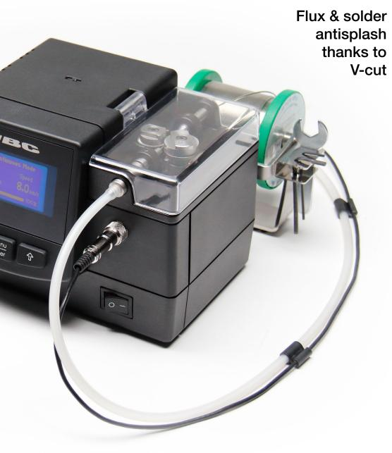
The blade perforates solder wire down to the flux core while feeding it.
