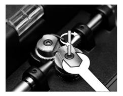
2. Replace the wheel, the blade clamp and the blade with the new ones.
