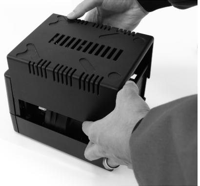
To have access to the connection you need loose the screws and release the frontal part carefully
