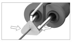
Pinch the wire with the blades acording to the diameter of the wire to be stripped. The pinched area will be melted by heat.
