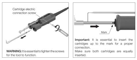
W440 cartridges have a proper centering to ensure a good functionality.
