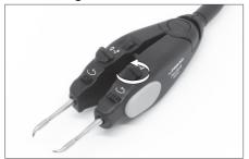
Unlock the fixing knobs.
