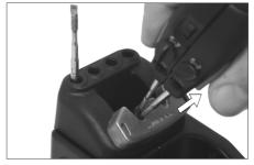
Place the cartridges in the extractor and pull the tweezers to remove them.
