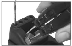
Use the grooves to insert the cartridges as far as they stop.
