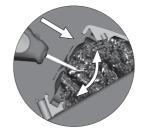
If the tip is very dirty, JBC recommends first cleaning it with the wiper to remove excess solder.
