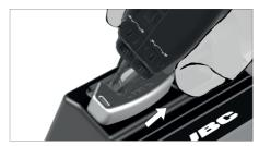
Place the cartridges in the extractor and pull the tweezers to remove them.
