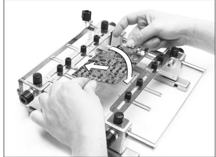
Push the PCB against the SP guide, position it and tighten the SP guide knobs.
