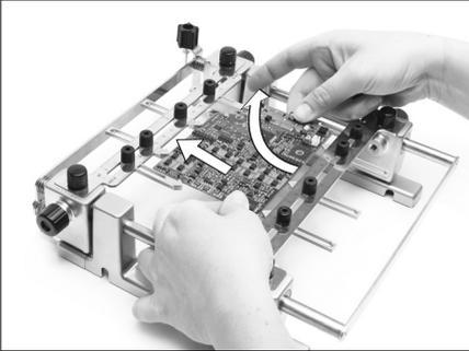
After loosening the SP guide knobs, push the PCB against the SP guide and lift out.
