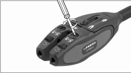
Unlock the fixing screws.
