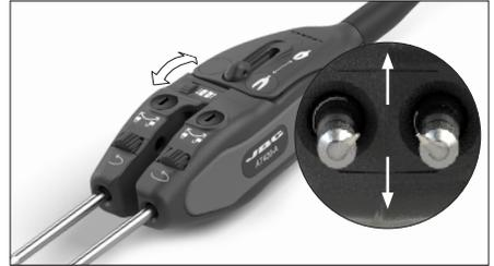
The rear wheel allows the cartridges to be equally aligned when you close the tweezers.
